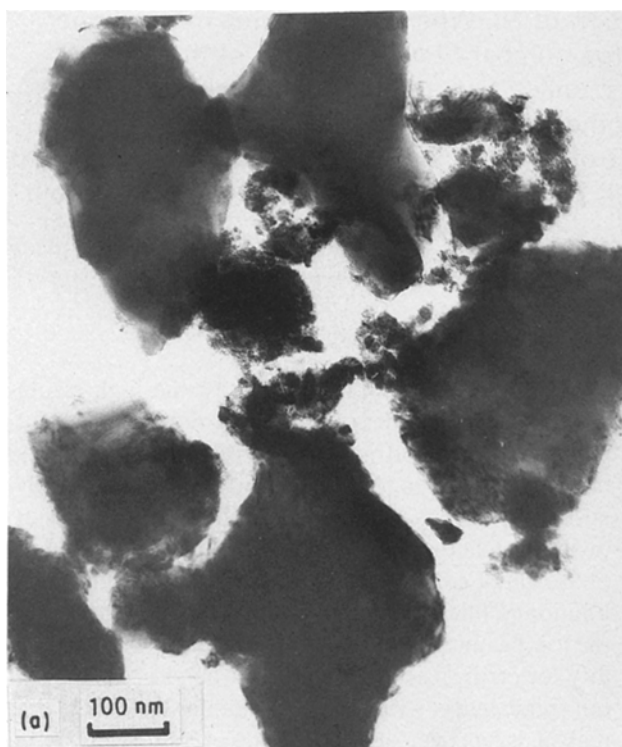
Figure 2 TEM (a) bright- and (b) dark-field imaging of ground nickel–alumina powder used for hot-pressing. Some of the Ni powder is contrasted, showing an extremely good dispersion of Ni powder among the much larger transition alumina grains.
